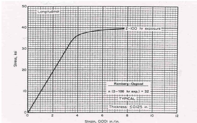
Figure 2. Tensile stress-strain curve of Aluminum alloy 6061-T6
